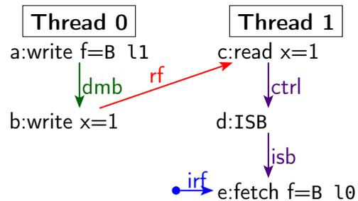
This test includes sufficient synchronisation on each thread to enforce thread-local ordering of data accesses: the **DMB** in Thread 0 ensures the writes **a** and **b** propagate to memory in program order, and the control-dependency into an **ISB** on Thread 1 ensures the read **c** and the fetch **e** happen in program order. However, as we saw in §2, this is not enough to synchronise concurrent modification and execution of code in ARMv8-A. Thread 0 needs the entire
