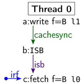
Now the outcome is forbidden. The cache synchronisation sequence **DC CVAU; DSB ISH; IC IVAU; DSB ISH** (which we abbreviate to a single **cachesync** edge) ensures that by the time the **ISB** executes, the instruction and data memory have been made coherent with each other for **f**. The **ISB** then ensures the final fetch of **f** is ordered after this sequence. The microarchitectural intuition for this was in §2; our §4 operational model will describe the semantics of each instruction.
