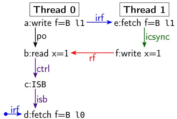
**f**, Thread 1 fetches the new value and performs just an **IC** and **DSB**, before signalling Thread 0 which also fetches **f**. That **IC** is not strong enough to ensure that the write is pulled into the instruction cache of Thread 0.
